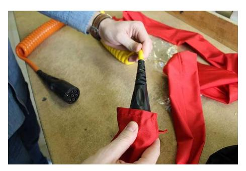
3. Pull the cover over the entire cable and insert the fixing strips through the loops.
