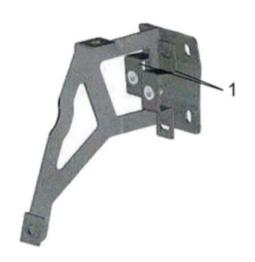
1. remove the acrylic part from the brackets Attach the light struts to the middle brackets as shown in the drawing with M6x25mm hexagonal screws.
