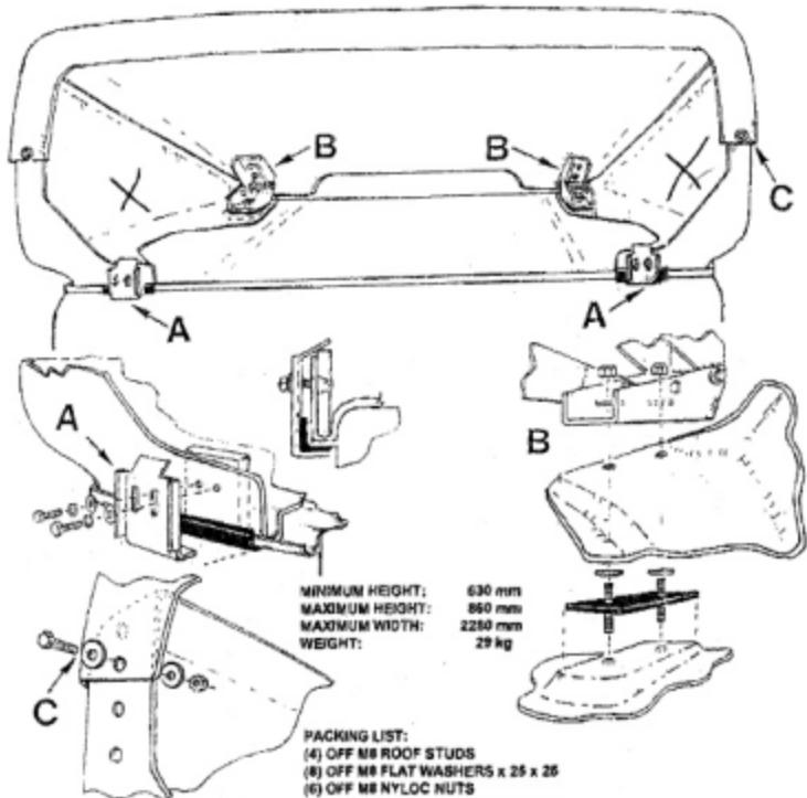
1. Drill out the 4 raised bumps towards the front of the cab. Screw the 4 M8 studs into captive nuts, (long end first).
